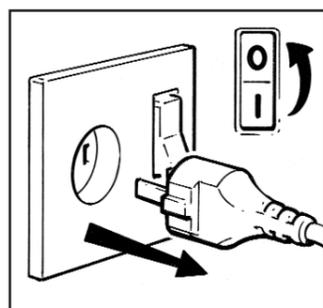
Switch off the drinks station and disconnect from the mains power supply.
