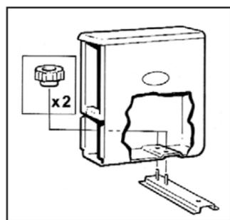
Attach the metal bracket using 2 plastic thumbnuts.
