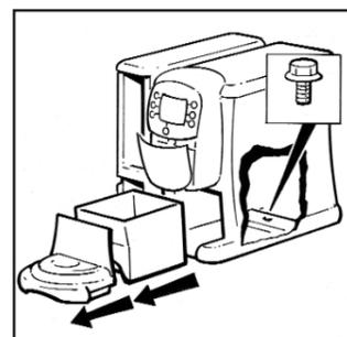
Remove the drip tray and pack bin from the Drink Station And secure the metal brace with the large nut.
