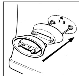
Slide the two spacer brace parts onto the long bolts.
