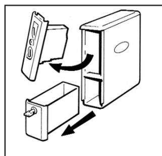
Using the key supplied remove the interface panel and cash box.
