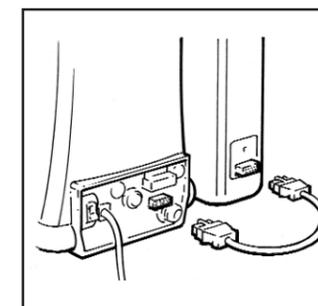
Connect the Pay Module to the Drinks Station with the cable. Re-assemble the Pay Module and Drink Station.
